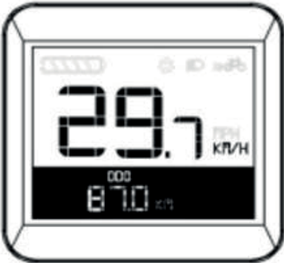
Real time speed ,accumulative mileage
